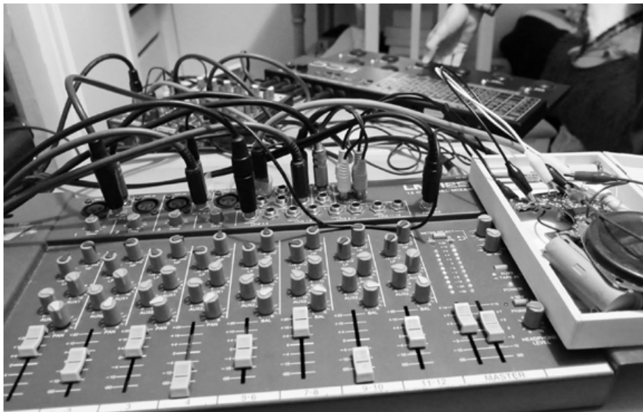
Example of feedback in a audio mixing console, connecting the outputs into the inputs.
